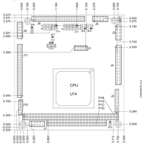
Figure 2-7. Mechanical Dimensions (Top View)
